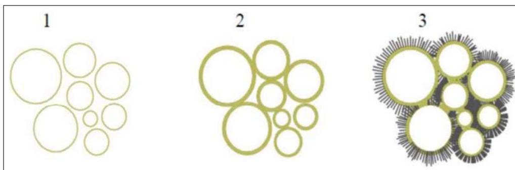
**Fig. 1.** Cross-section of cement grains to represent the hydration stages in Portland cement [7]. 1. Before contact with water, 2. shortly after contact with water (C-S-H gel around the grains and long thin ettringite needles), 3. intertwining of the needles and continuation of hydration by joining all the components of the phases
