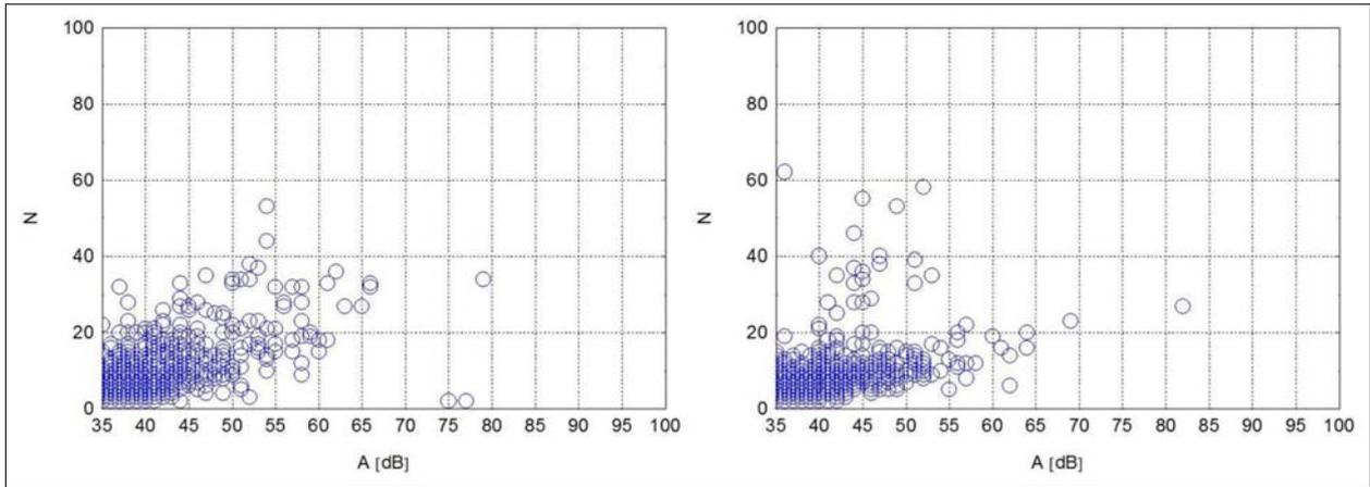
Fig. 6. Comparison of the dependence of the number of events on the amplitude (composite A – left, composite B – right)
