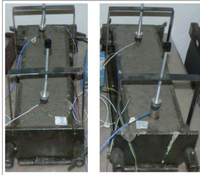
Fig. 2. Photographs from the production with the layout and details of distribution of the AE sensors (composite A (left), composite B (right))
