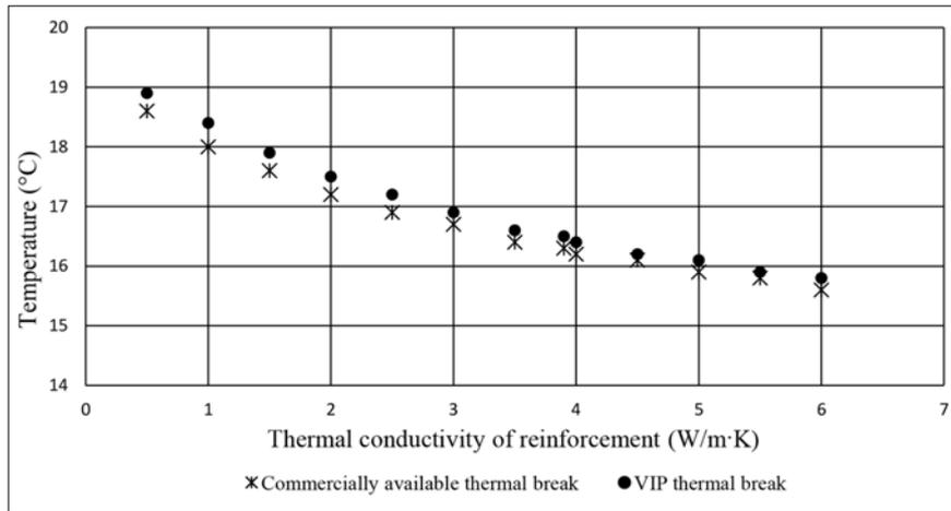
**Fig. 5.** Comparison of thermal effectiveness of various reinforcement bar conductivity in commercially available and hybrid thermal break
