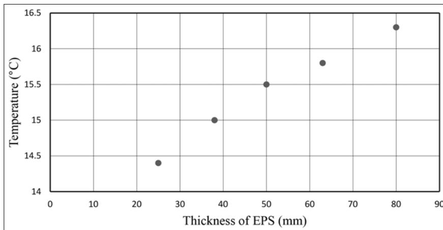
**Fig. 6.** The effect of the thickness of EPS thermal break on temperatures at the ceiling-wall junction
