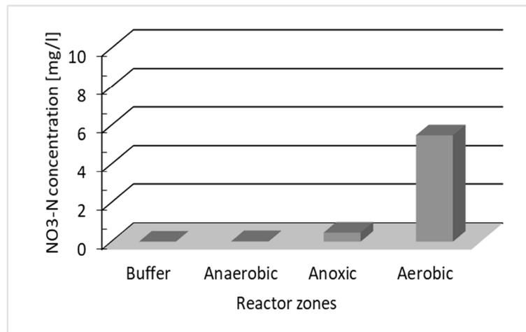
Fig. 4.  $\text{NO}_3\text{-N}$  concentration in the reactor zones
