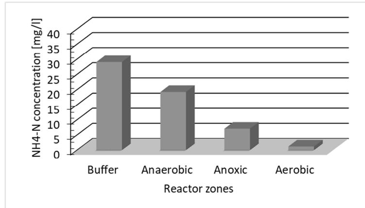
Fig. 3.  $\text{NH}_4\text{-N}$  concentration in the reactor zones
