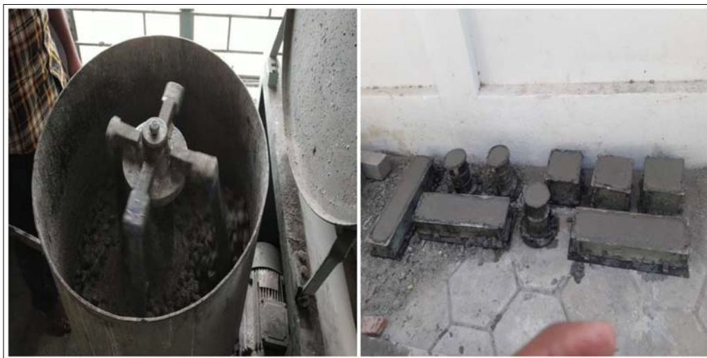
Fig. 1. Casting of concrete specimens
