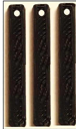
Fig. 6. The printed fatigue specimen from a carbon fiber filament
