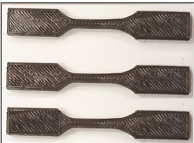
Fig. 4. The tensile specimen was printed from a carbon fiber filament
