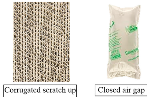
Fig. 1. The types in filling hollow of the studied building blocks 'Source: Author'
