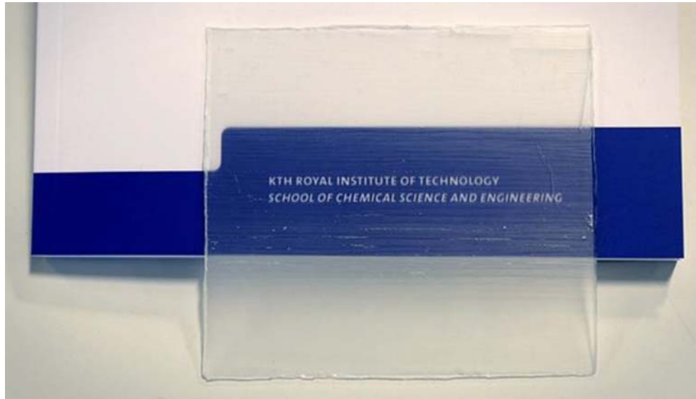
Fig. 1. Transparent wood sample created at KTH [1]
