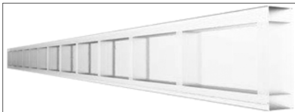
Fig. 5. Transparent wood Vierendeel box beam – rendering
