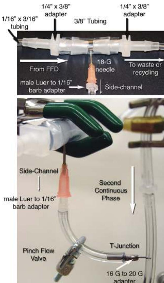
Figure S1. Photographs of the particle concentrator device and side channel with fittings and tubing labeled.
